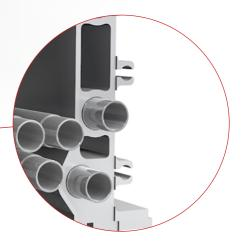
A carefully engineered hydroforming process fixes the cooling tubes inside the sidewalls, providing the highest possible thermal conductivity.
